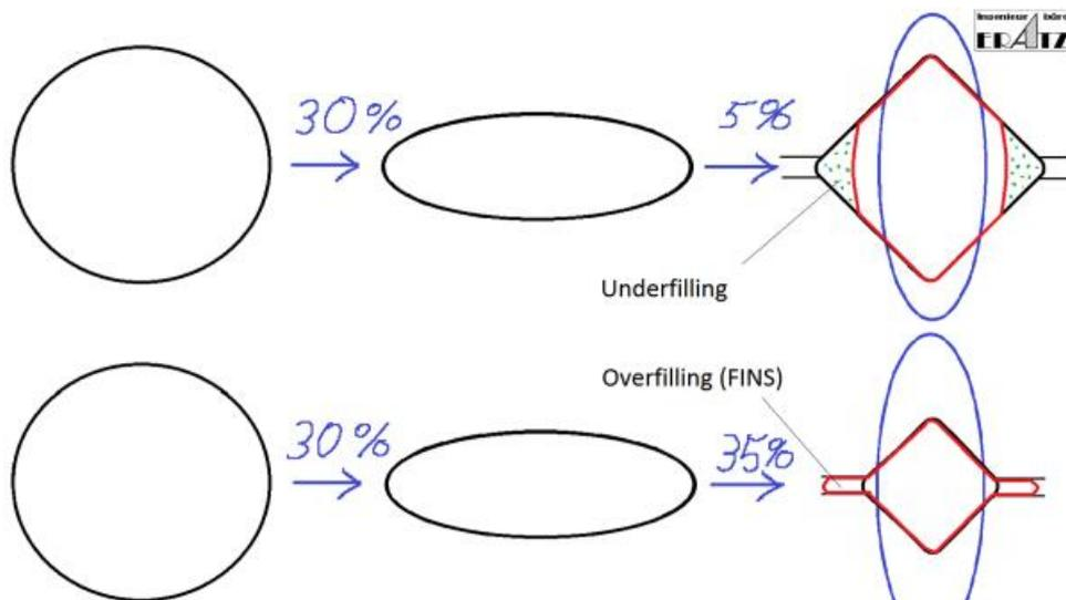
For steel material the rule for linked reduction in the non-spreading cross-section is as follows:
